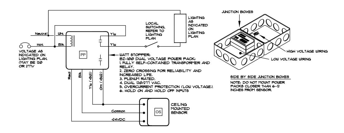
OCCUPANCY SENSOR WIRING DIAGRAM E402 SCALE: NONE
