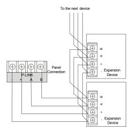
RA-6500R Class A Wiring Example Fig 2
