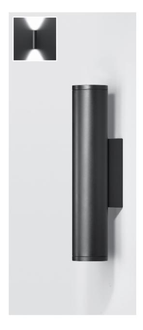
Housing: Constructed of copper free die-cast aluminum alloy. The housing uses stainless steel inserts for enclosure attachment. Mounts over a standard 3½" or 4" octagonal wiring box. Die castings are marine grade, copper free (≤ 0.3% copper content) A360.0 aluminum alloy.
