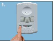
Push and hold the Test/Hush button for two seconds to enter RealTest mode. The green LED will flash once every second to indicate RealTest mode has started.
