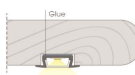
G Recessed Mounting into a Mitered Groove using a flanged Channel
