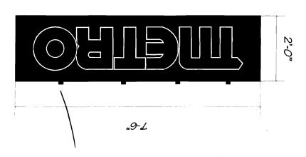
Plate w/4 holes each drilled shielded 3/8 x 2 1/2" Bolt 16 total.
