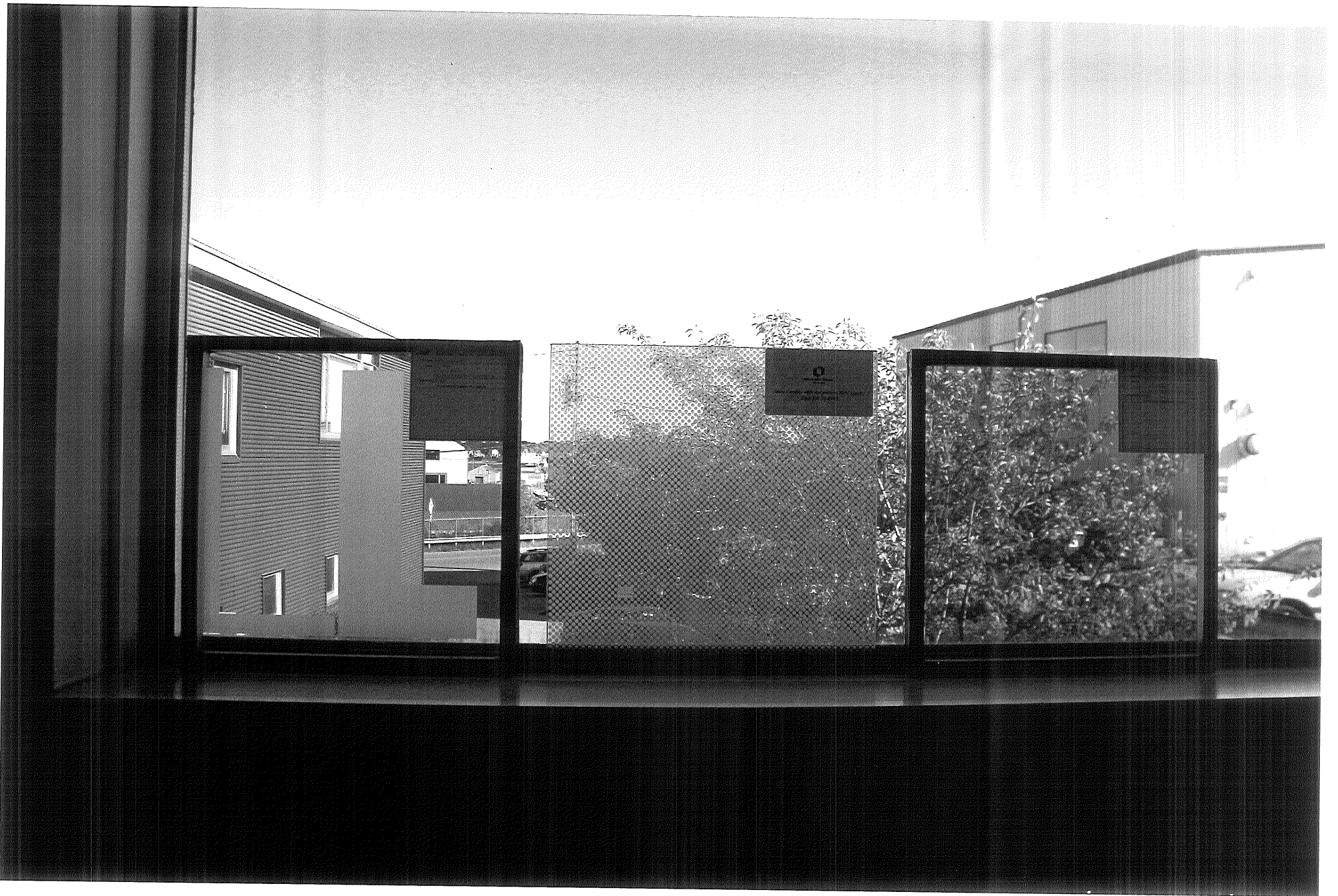
Glass Samples From left to Right : ① 3M Vinyl Lettering ② Fritted Glass ③ Clear Glass
