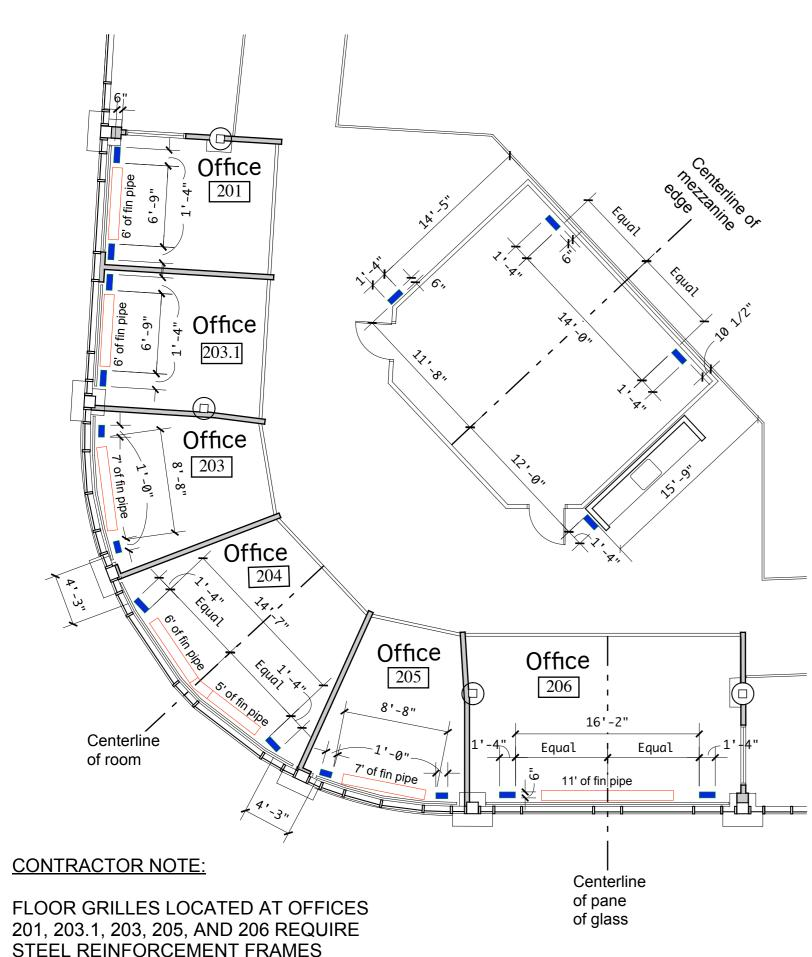
201, 203.1, 203, 205, AND 206 REQUIRE STEEL REINFORCEMENT FRAMES PER SKS 32 DATED 9/28/09.
