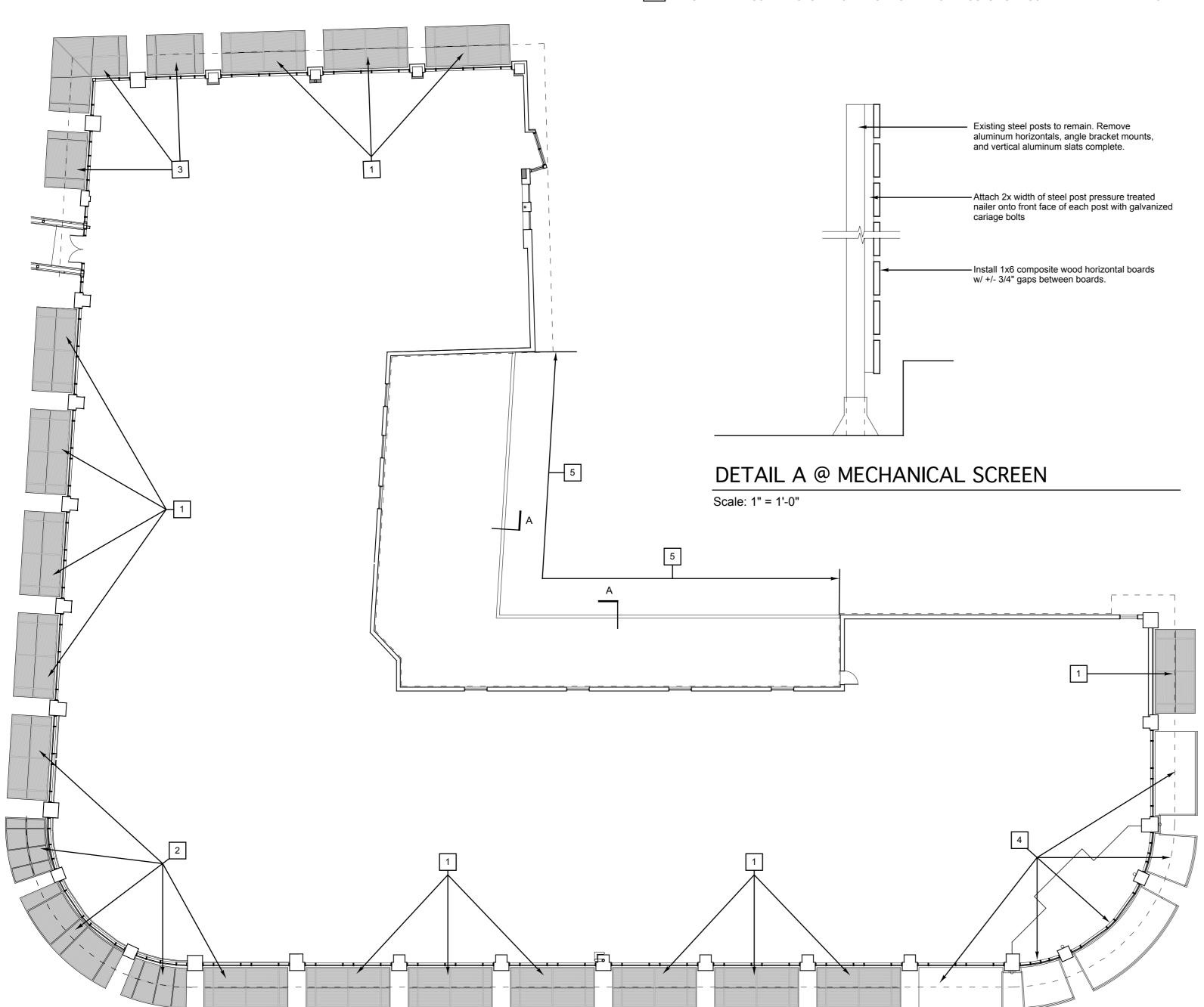
KEY PLAN FOR REPAIRS AND MODIFICATIONS TO EXISTING CANOPIES & MECHANICAL SCREEN
