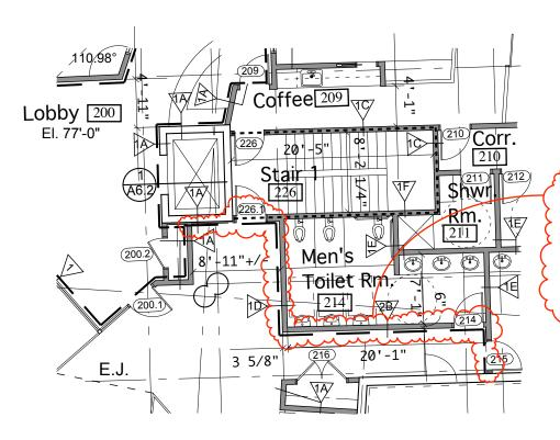
The partitions indicated are smoke partitions. Extend up to underside of deck and seal all penetrations. Doors 214 & 215 shall have a 20 minute rating with closers and smoke seals.
