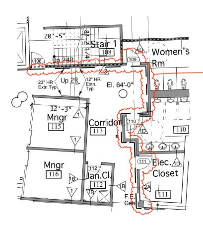
The partitions indicated are smoke partitions. Extend up to underside of deck and seal all penetrations. Doors 109, 110, & 111 shall have a 20 minute rating with closers and smoke seals.
