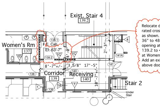
Relocate door 139.2 into new 1 hour rated cross corridor partition type1C as shown. Change door width from 36" to 48". Enlarge doorway opening at former location of door 139.2 to 48" wide. Revise partition at Women's Room to be1 hr. rated. Add an exit sign at corridor 139 above door 139.2
