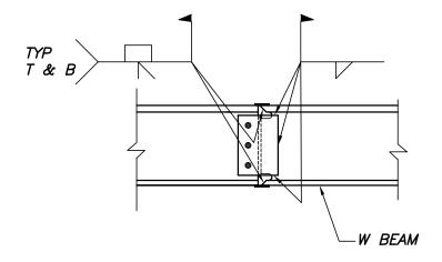
NOTE: SPLICE SHALL OCCUR WITHIN MID 1/3 OF OVERALL BM SPAN. INSTALL BM SUCH THAT TOP FLANGE IS SNUG TO UNDERSIDE OF FLOOR DECK, TYP.
