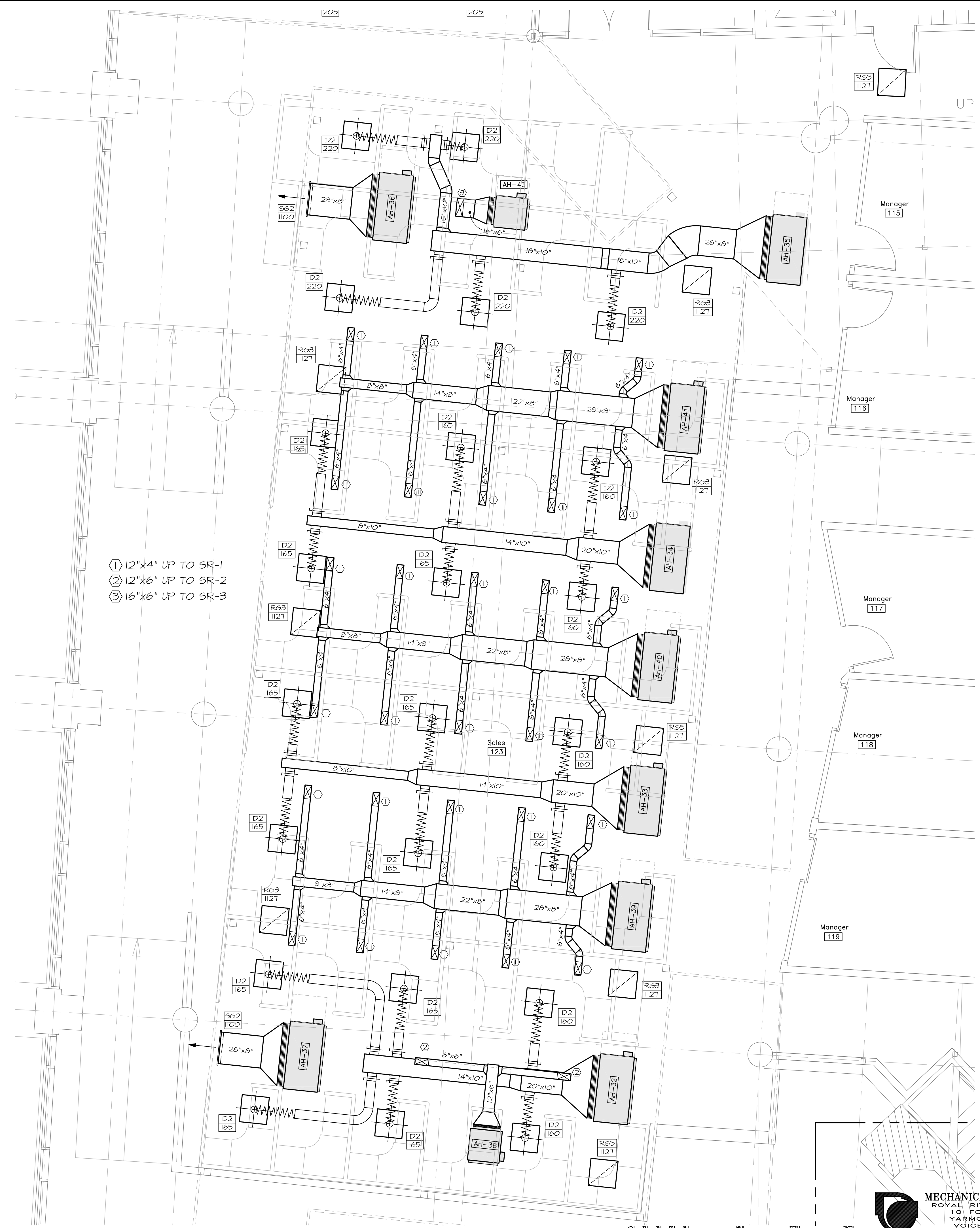
SECTION AT AIR HANDLERS 13, 21, 23, 24, 36 & 37 SCALE: 1/2" = 1'-0"
