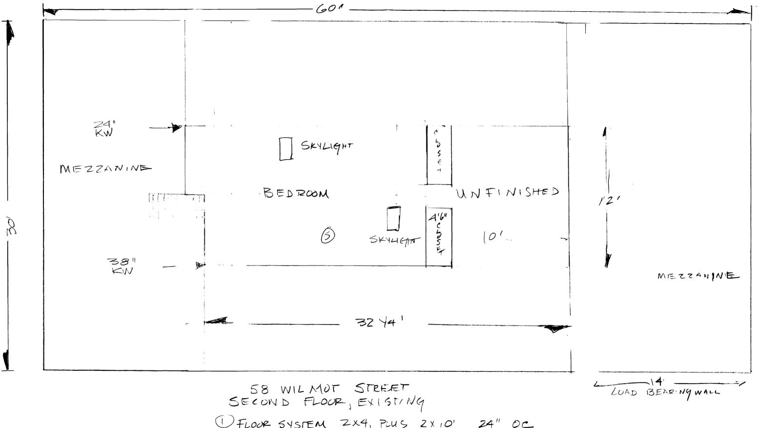
THOOR SYSTEM ZX4, PLUS ZX10' 24" OC 2) ROOF RAFTERS ZX8 (ROUGH) Z4" OC 3) FLOOR SHEATHING DOUBLE LAYER Y2" 418 PLYWOOD 4) ROOF 12X12 PLTCH
