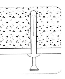
ZAMAC HAMMER SCREW" DRIVE ANCHORS AS MFG BY POWERS FASTENERS, NEW ROCHELLE, NY OR EQUAL:
