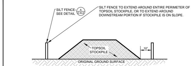
**TEMPORARY TOPSOIL STOCKPILE DETAIL**
