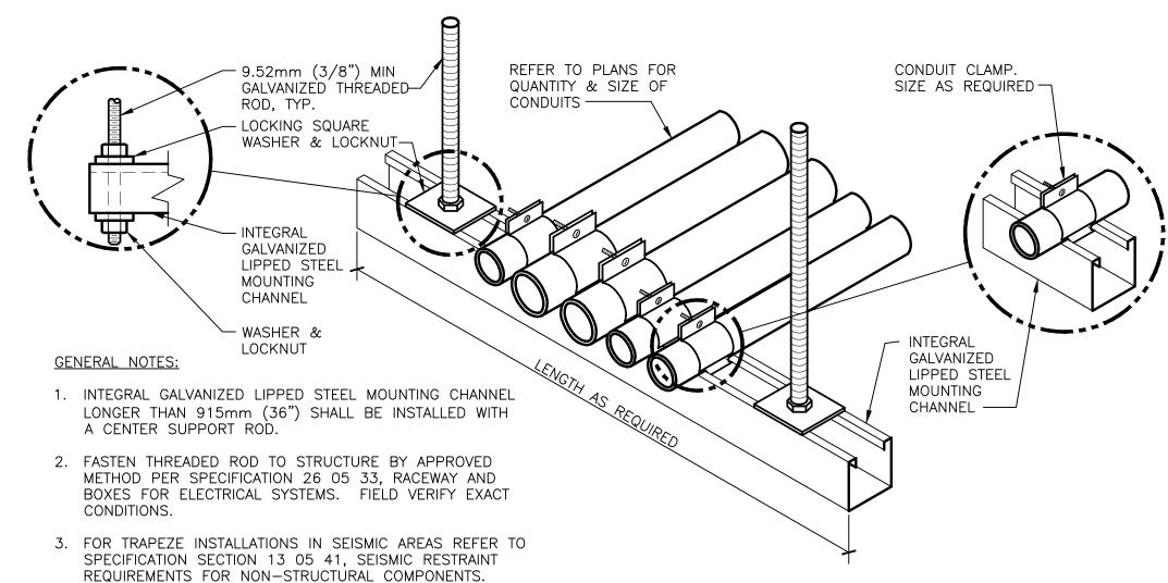
CONDUIT TRAPEZE MOUNTING DETAIL
