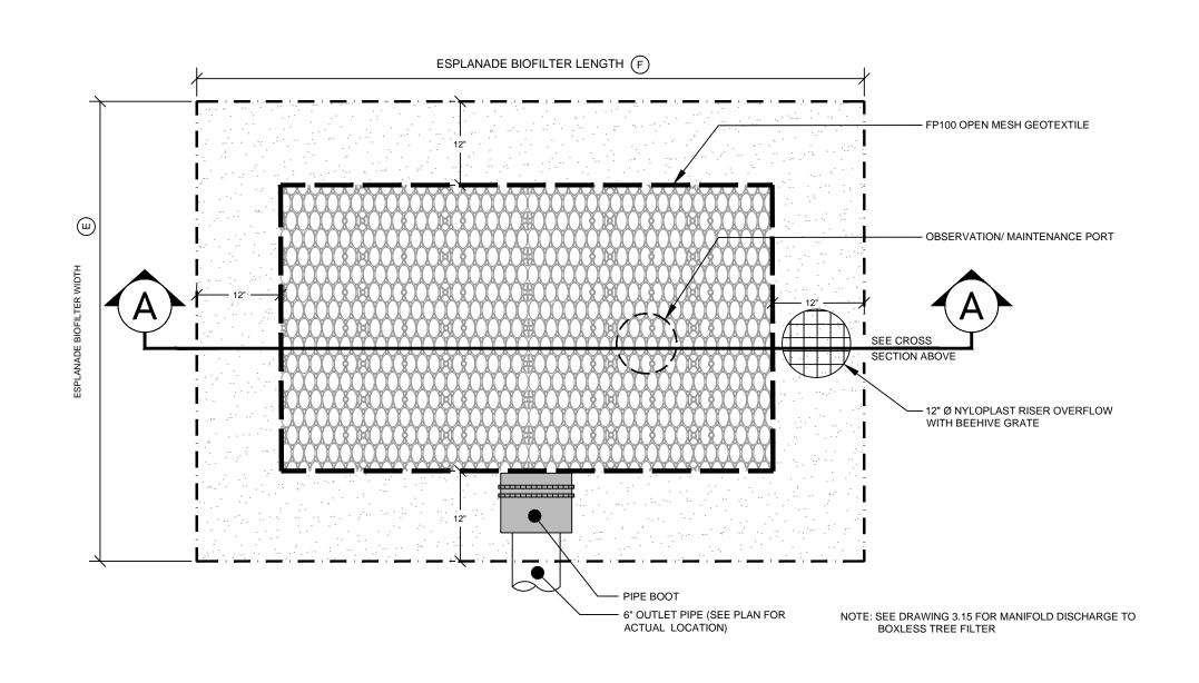
PIPE BOOT - FP100 OPEN MESH GEOTEXTILE STRUCTURAL UNDERDRAIN OBSERVATION PORT CONNECTION
