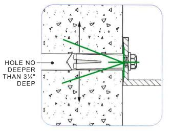
LOK-BOLT™ ANCHORING SYSTEM AS MFG BY POWERS FASTENERS, NEW ROCHELLE, NY OR EQUAL:
