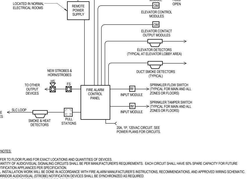
MINIMUM CONDUIT SIZE SHALL BE 3/4" RIGID CONDUIT. AND CITY. ALL CIRCUITS SHALL BE CLASS B LOOPS.
