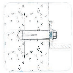
SLEEVE-ANCHOR MOUNTING DETAIL NOT TO SCALE
