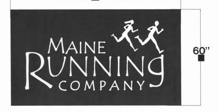
This will be an 8 inch deep Illuminated Sign Cabinet built to UL standards. The material will be standard extruded aluminum painted with polyurethane paint
