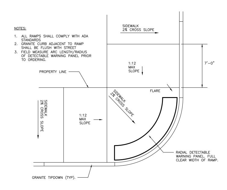
DIAGONAL SIDEWALK RAMP LAYOUT AT INTERSECTION FOR SIDEWALK WITHOUT ESPLANADE
