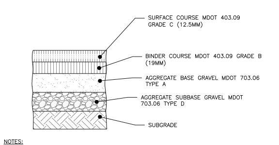
1. COMPACT SUBGRADE TO 95% MAXIMUM DRY DENSITY IN ACCORDANCE WITH ASTM D-1557. 2. ARTERIAL BITUMINOUS PAVEMENT PROFILE APPLIES ONLY WITHIN ANDERSON STREET R.O.W.
