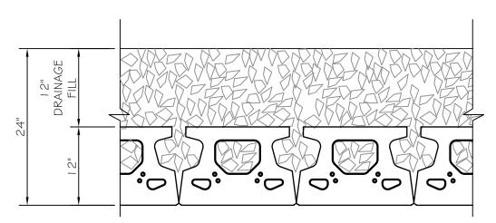
CRUSHED STONE UNIT COMPACT WITH HAND OPERATED PLATE COMPACTOR FILL ALL VOIDS INCLUDING PIN HOLES AFTER BLOCKS ARE ALIGNED. ALIGN EACH BLOCK COURSE PRIOR TO PLACING
