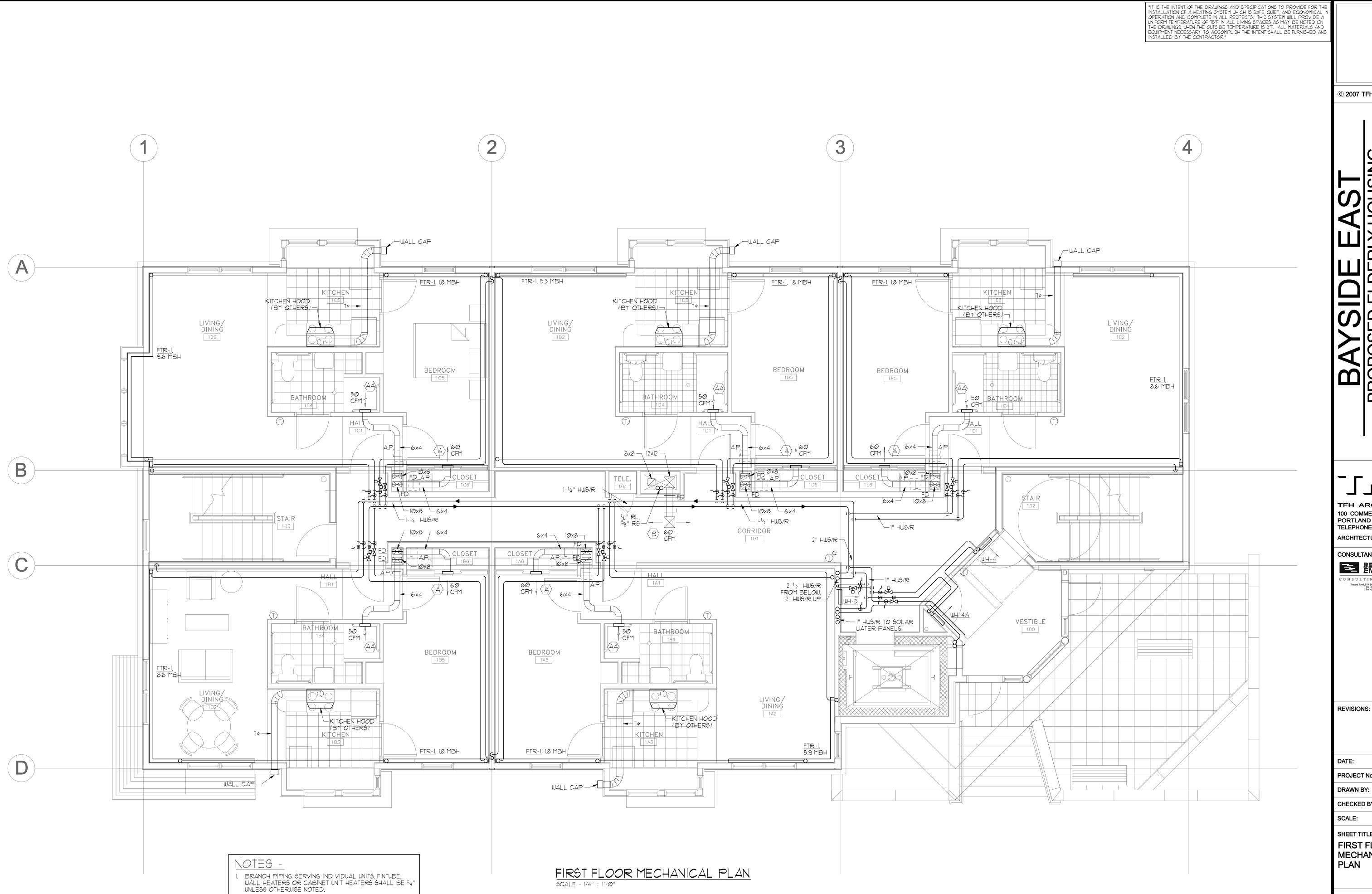
2. DUCTWORK IN UNITS SHALL BE INSTALLED IN SOFFITS BELOW THE RATED CEILING ASSEMBLY.
