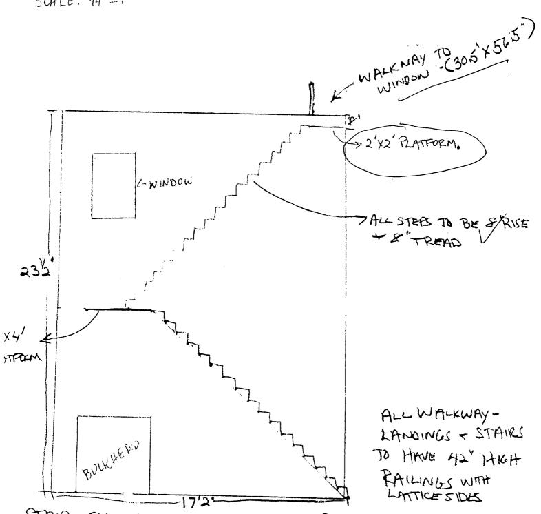
STAIR STRINGERS SHALL BE COT FROM 2X12 STOCK Treads to be steel 93/4w, linck thick, 24" long 4. DETAILS FOR MATTICE WITH HOREZ FRE HAM STANKI AT 161 CUMBERLANT AND PTLO, ME 4 59 WILL PROJECT HAMPIGATE WILL BE 1/2 "
