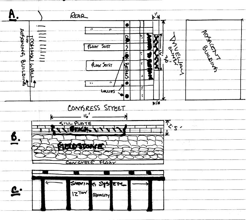
SCOPE: REMOVE CHANGED MASONING / EXCAVATE domo hate / want Share up flooring / Beams / Replace changed area with NEW 8" Black / Rebair / GOUTED WATER PROPER PROPER AREAS DATION: Replace Sun plate, if chemical NEW STARRY / P/TREATED
