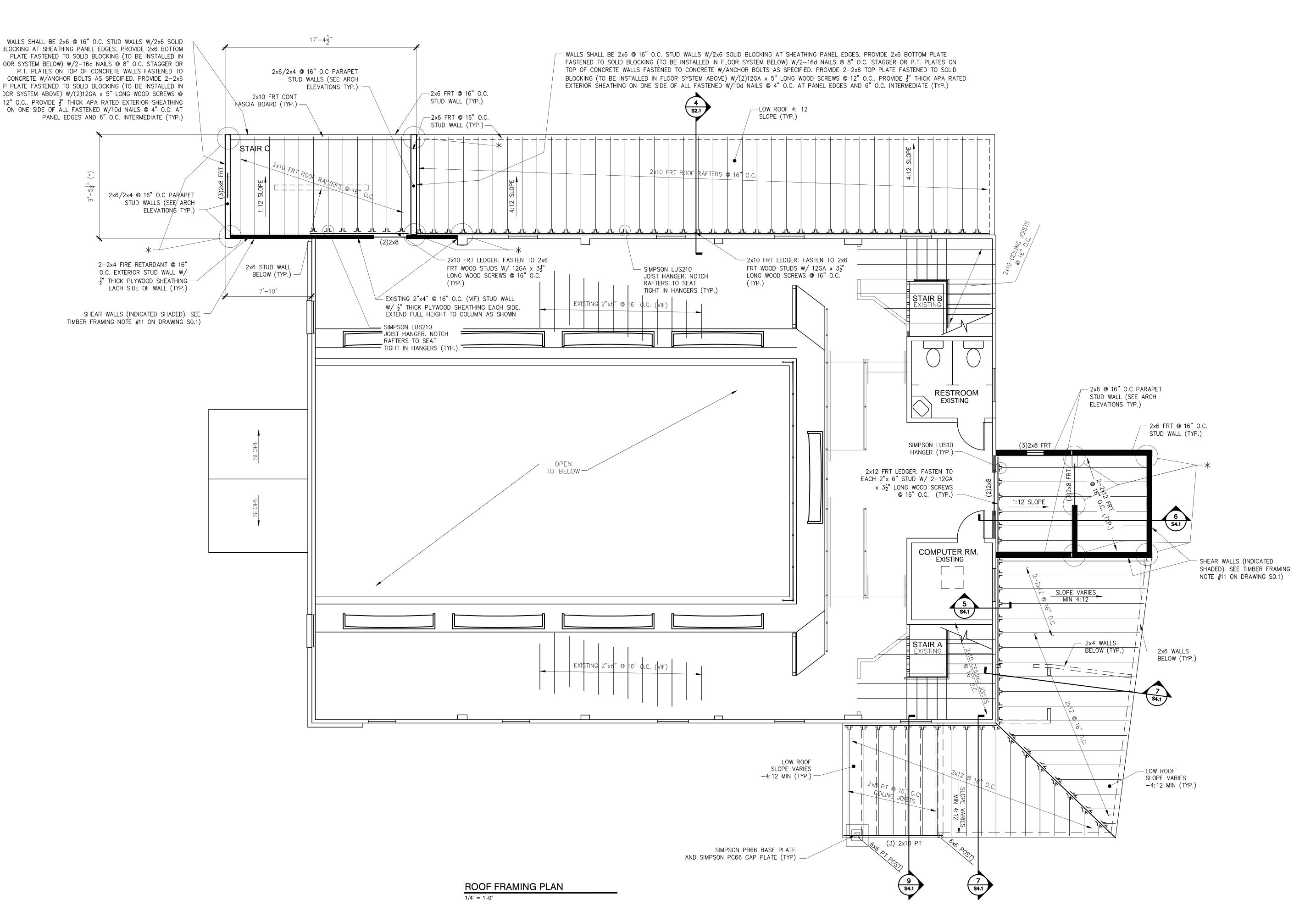
" $\star$ " indicates: post and hold down - see timber framing note #12 on drawing so.1
