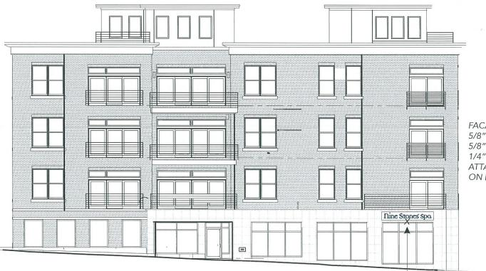
FACADE NOTES: 5/8" PYLWOOD 5/8" CEMENT BOARD 1/4" GRANITE VENEER ATTACHMENT TO BE ON MORTAR SEAMS
