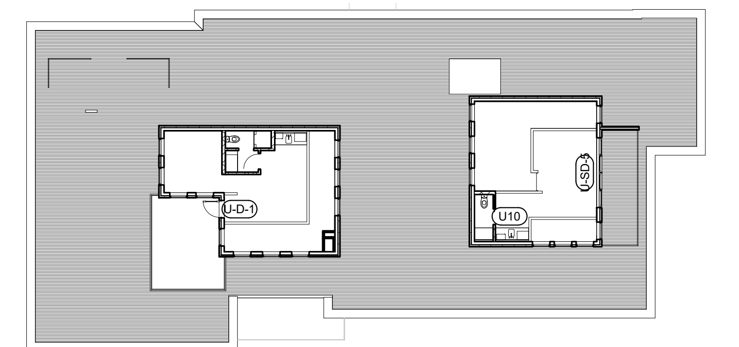
10 ROOF AND MEZZANINE DOOR PLAN 1/16" = 1'-0"
