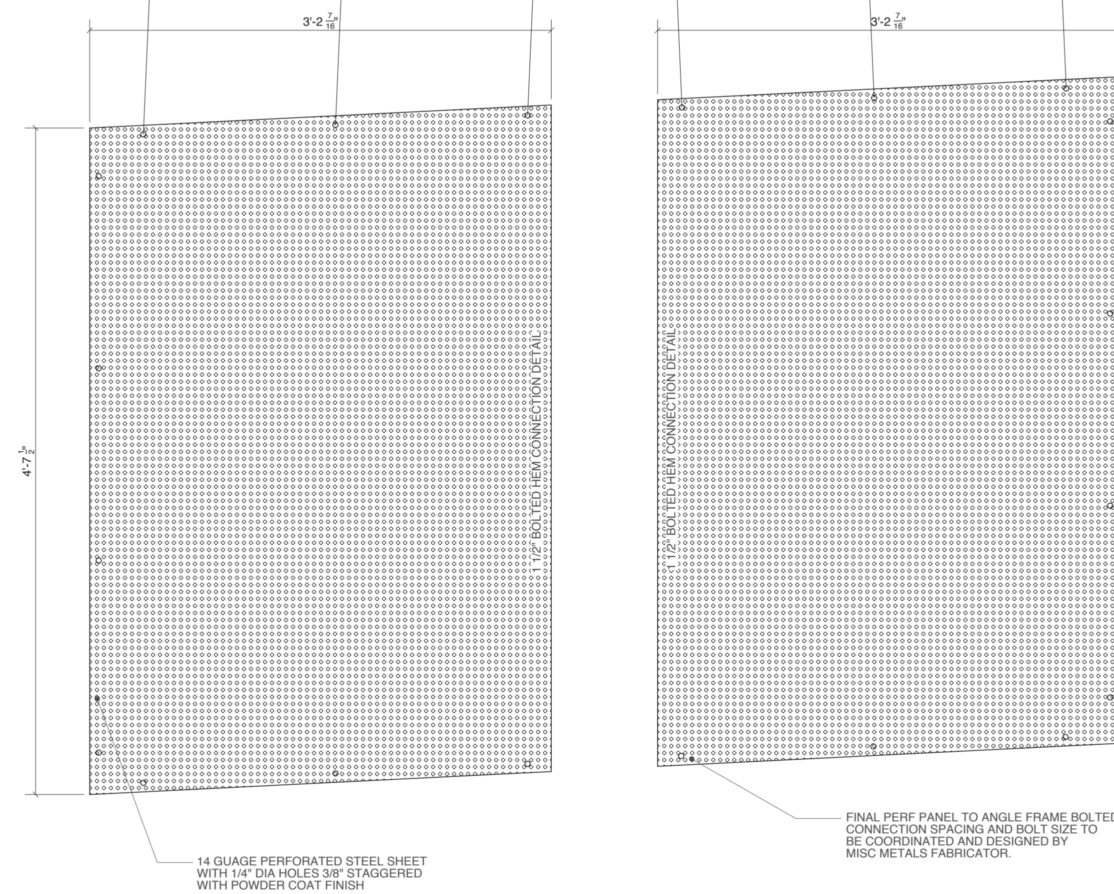
7 GUARD RAIL PANEL ELEVATION SCALE : 1 1/2" = 1'-0"
