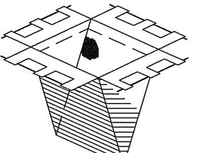
PRIOR TO FINAL GRADING AND PAYING OPERATIONS BEGIN A CATCH BASIN INSERT (SUCH AS A SILT SACK OR A DANDY BAG II) MUST BE INSTALLED IN EACH BASIN PER MANUFACTURES INSTRUCTIONS, HAY BALES SHOULD BE REMOVED ONCE INSERTS ARE INSTALLED.
