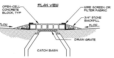
ELEVATION 5 BLOCK SEDIMENT BARRIER
