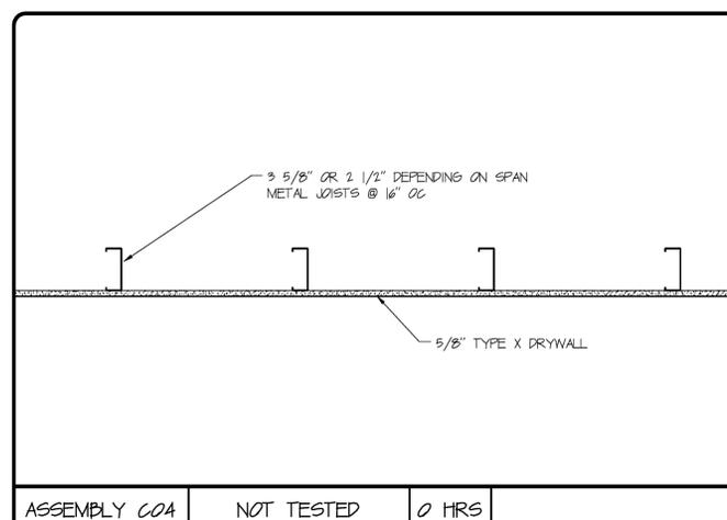
ASSEMBLY C04 NOT TESTED 0 HRS
