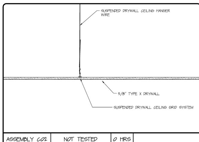
ASSEMBLY C02 NOT TESTED 0 HRS
