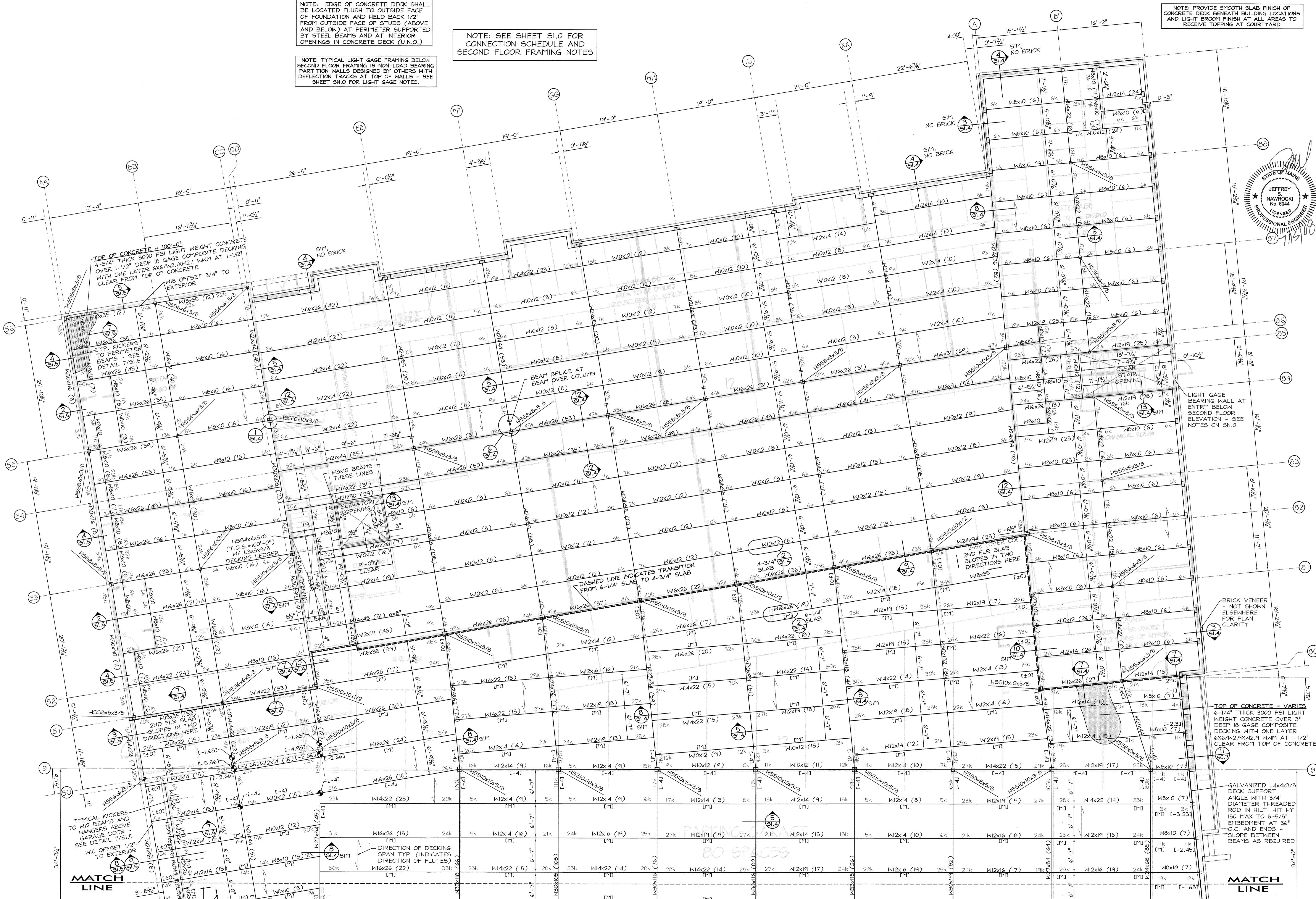
SECOND FLOOR FRAMING PLAN 1 - BUILDING 2 S1.1 Scale: 1/8" = 1'
