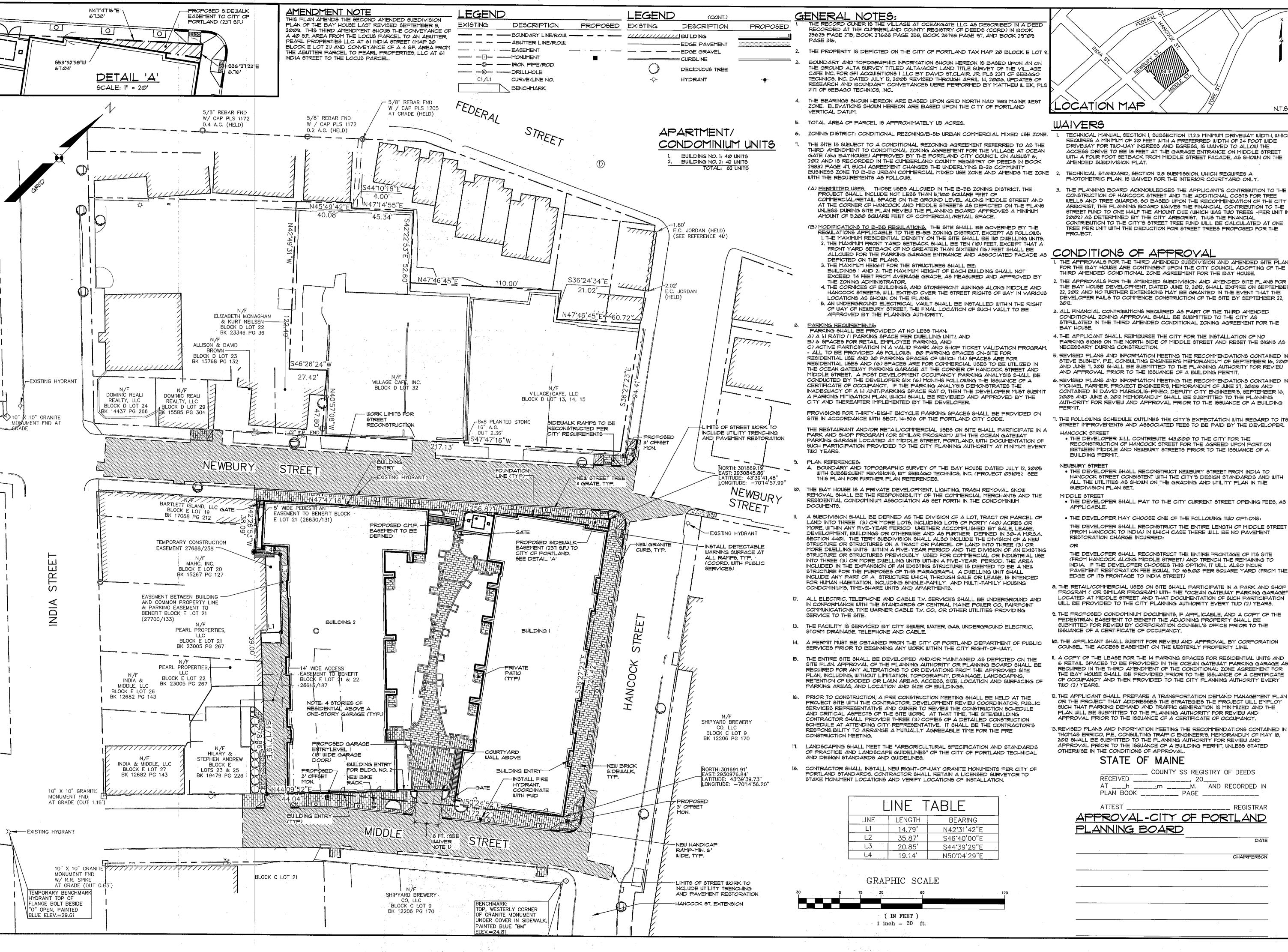
TECHNICAL MANUAL, SECTION 1, SUBSECTION 1.1.2.3 MINIMUM DRIVEWAY WIDTH, WHICH REQUIRES A MINIMUM OF 20 FEET WITH A PREFERRED WIDTH OF 24 FOOT WIDE DRIVEWAY FOR TWO-WAY INGRESS AND EGRESS, IS WAIVED TO ALLOW THE ACCESS DRIVE TO BE IS FEET AT THE GARAGE ENTRANCE ON MIDDLE STREET WITH A FOUR FOOT SETBACK FROM MIDDLE STREET FACADE, AS SHOWN ON THE
