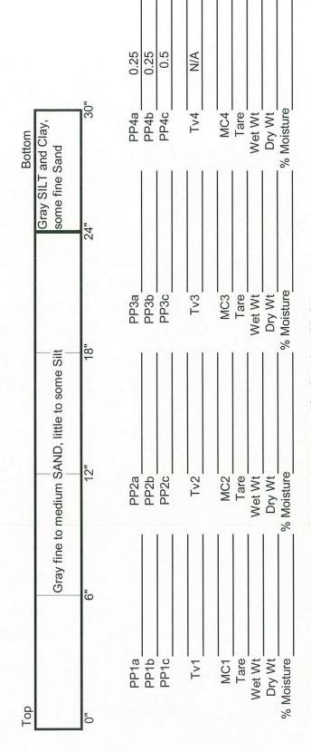
PP - Pocket Penetrometer TV- Torevane MC- Moisture Content
