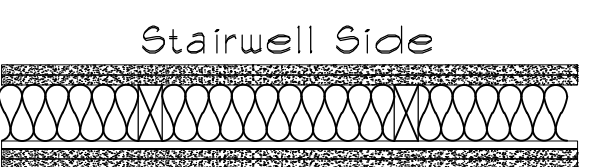
W3 1 Hour Wall Assembly 50-54 STC - UL 334 Gypsum Board, Wood Studs, Resilient Channels, Insulation
