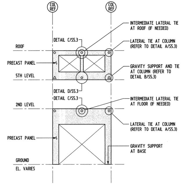
**TYPICAL PRECAST PANEL ELEVATION**
