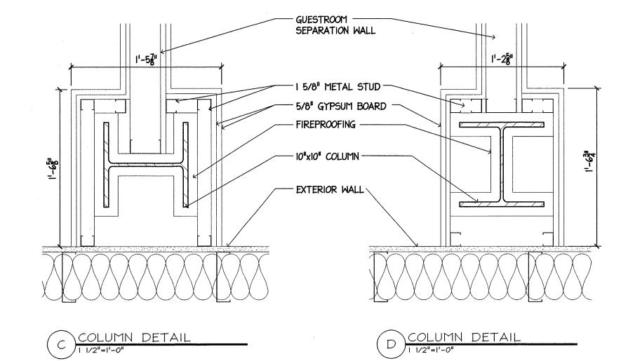
To maintain integrity of fire rating and STC on demising wall finish material must wrap column. Follow profile of column as required. Column placement may vary.
