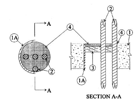
1. Floor or Wall Assembly-Min 4-1/2 in. thick lightweight or normal weight (100-150 pcf) concrete. Wall may also be constructed of any UL
