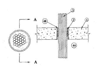
1. Floor or Wall Assembly - Min 4-1/2 in. thick reinforced lightweight or normal weight (100-150 pcf) concrete. Floor may also be constructed of any min 6 in. thick UL classified hollow-core Precast Concrete Units\*. Wall may also be constructed of any UL Classified Concrete Blocks\*. Max diam of opening
