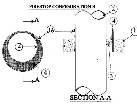
Floor or Wall Assembly — Min 2-1/2 in. thick lightweight or normal weight (100-150 pcf) concrete. Floor may be constructed of any min 6 in. thick UL Classi ed hollow core Precast Concrete Units\*. Wall may also be constructed of any UL Classi ed Concrete Blocks\*. Max diam of circular through opening is 10 in. See Concrete Blocks (CAZT) category in the Fire Resistance Directory for
