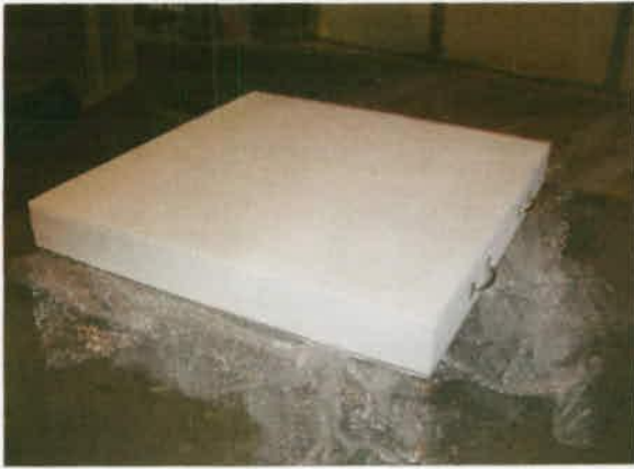
Before test: test sample ceiling, side to be exposed
