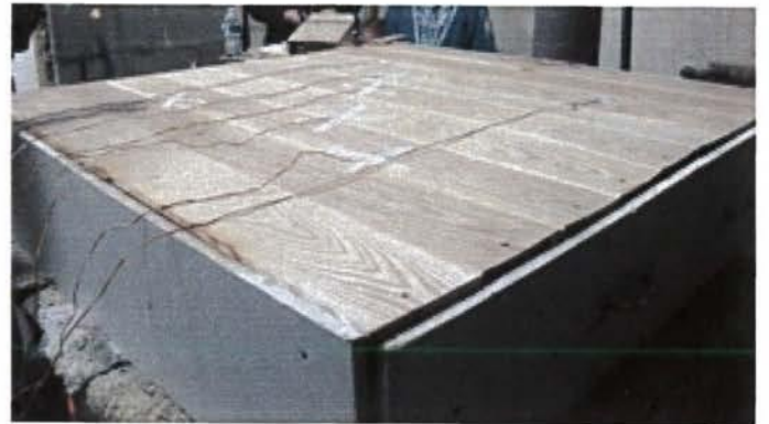
After test: unexposed side—no flame through
