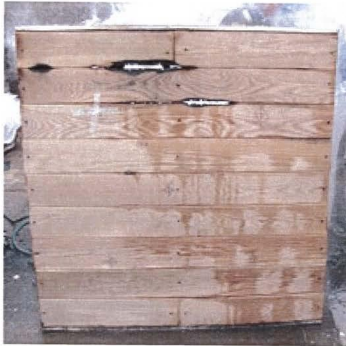
After test: unexposed side
