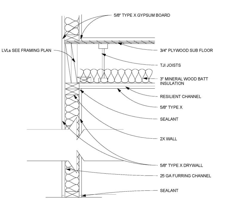
WALL ASSEMBLY BETWEEN EXIT ENCLOSURE AND DWELING UNITS NTS
