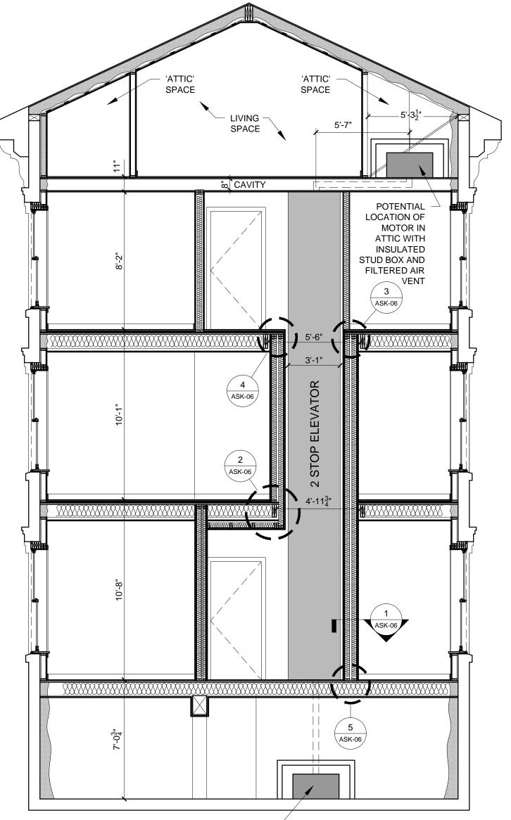
INSULATED STUD BOX AND FILTERED AIR VENT SECTION THROUGH ELEVATOR 6
