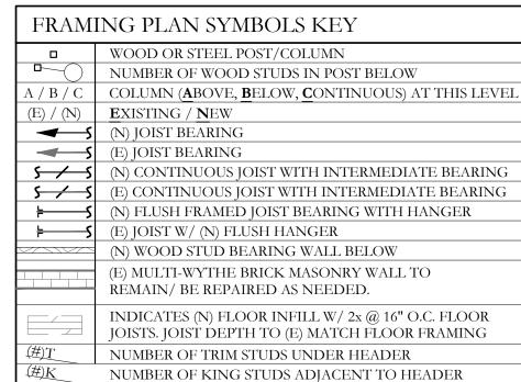
(N) CONTINUOUS JOIST WITH INTERMEDIATE BEARING (E) CONTINUOUS JOIST WITH INTERMEDIATE BEARING INDICATES (N) FLOOR INFILL W/ 2x @ 16" O.C. FLOOR
