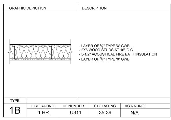
1.) REFER TO STRUCTURAL DRAWINGS FOR STUD SIZE AND SPACING
