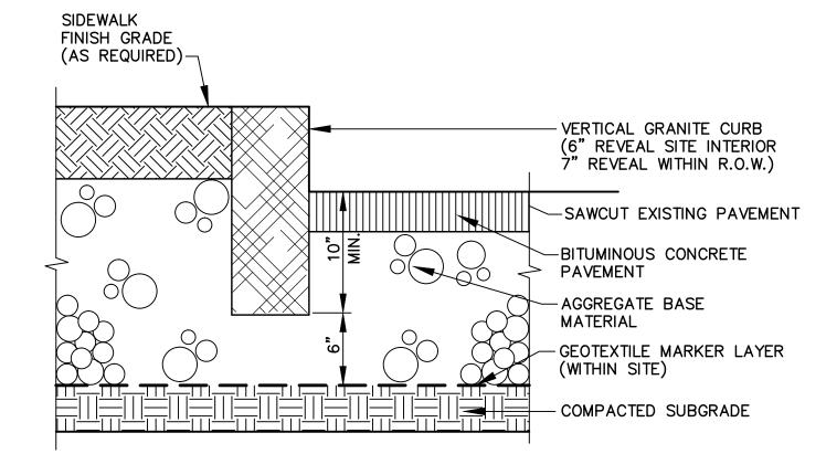
PAVEMENT DEPTH TO MATCH GREATER OF EXISTING PAVEMENT OR STANDARDS FOR CORRESPONDING STREET CLASSIFICATION
