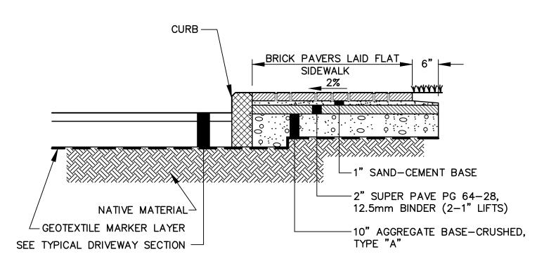
BRICK PAVER SIDEWALK SECTION (TYPICAL WITHIN SITE)
