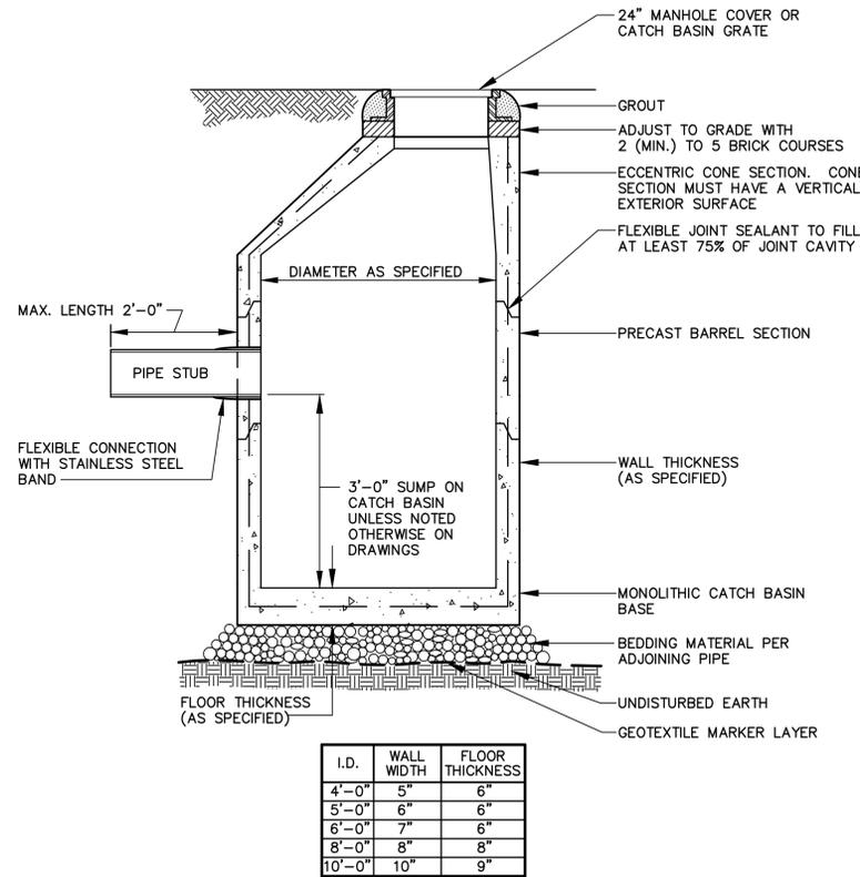
1 PRECAST CONCRETE MANHOLE
