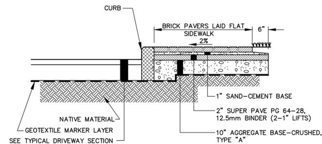
**6 BRICK PAVER SIDEWALK SECTION (TYPICAL WITHIN SITE)**
